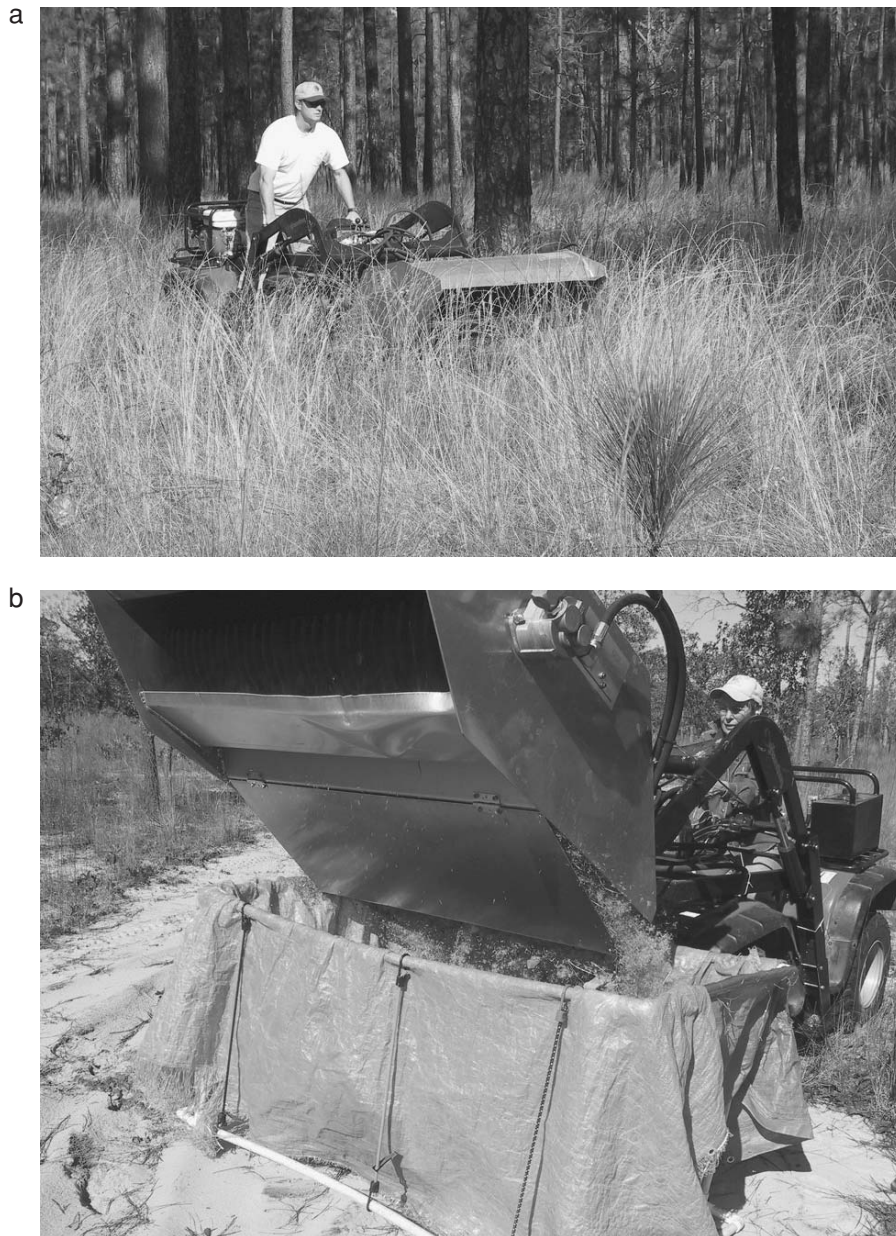
FIGURE 4. Bulk seed collection with an ATV mounted seed stripper in a remnant upland site (a) and emptying the collection hopper into a storage bin (b). Seed collections include seed from all species in fruit at the collection time, e.g., common large grasses and composites. (Photo courtesy of Lin Roth.)
