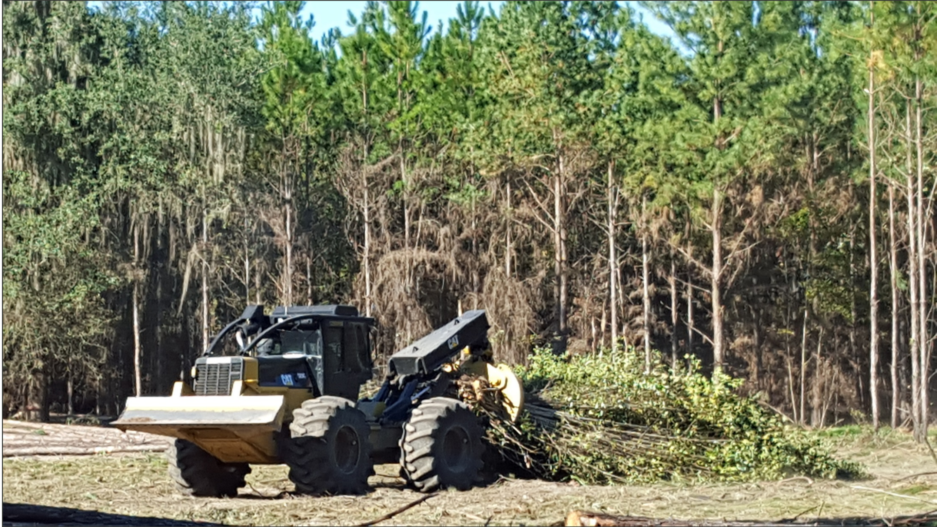
Separating the biomass from the pulpwood and chipping on site
